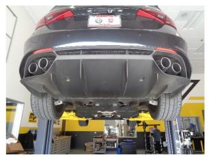
**Step 1**: Before extracting the OE exhaust system you will need to remove all the underbody covers as well as the cross member and rear valance. Also unplug the vacuum lines attached to both exhaust valves.
