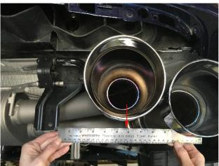
**Step 6.** Install the tips and roughly align them as follows: VERTICAL: align the TOP of the inner exhaust tips to 2 1/4" down from the seam between the bumper cover and the lower valence. HORIZONTAL: align the CENTER of the inner exhaust tips to 5 3/4" from the edge of the lower valence support located directly behind the exhaust mount. (See photos)
