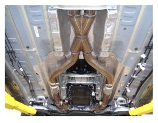
**Step 3.** Begin installation of the new system by loosely attaching the X-Pipe Assembly to the outlets using the Supplied 2.50 clamps and fitting the hangers into the insulators. Leave all clamps loose until final adjustment.
