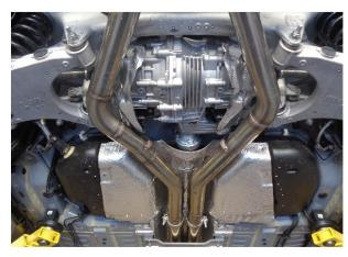
**Step 4.** Next, attach the Mid Pipe Assemblies to the X-Pipe Assembly using the supplied 3.00" clamps and fitting the hangers into the rubber insulators.
