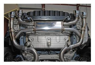
**Step 5.** Finish the initial installation by fitting the Muffler Assembly onto the Mid Pipe Assemblies using the supplied 3.00" clamps and inserting the hangers into the rubber insulators. Re-attach vacuum lines to valves, Attach extension hoses to vacuum lines and re-attach lines to the valves, and attach cross member.
